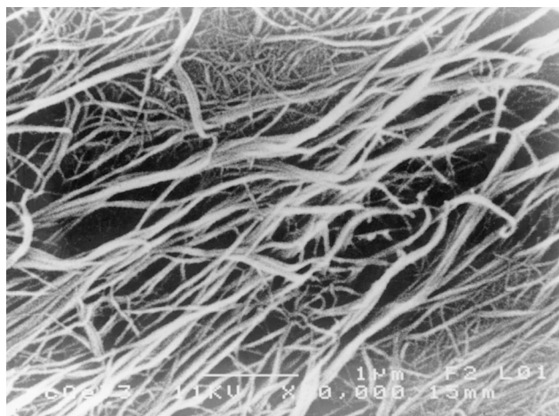
Figure 5. Scanning electron micrograph (SEM) of aerogel from 1 ( R^1 = p\text{-MeC}_6\text{H}_4 ).
